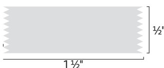
Figure 02 - Minimum size recommended for double-sided tape.
